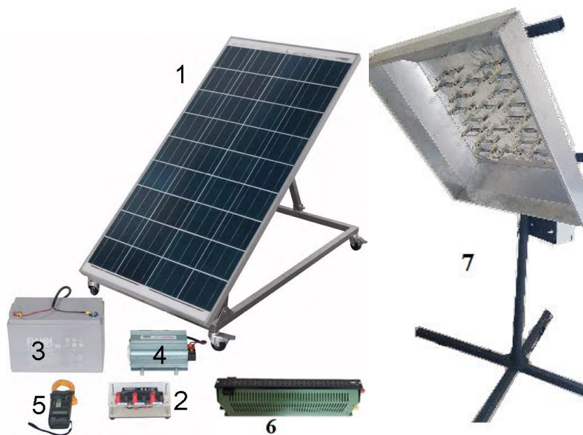
Fig. 8: (1) photovoltaic panel with variable, (2) solar charge controller, (3) storage battery inclination supporting structure, (4) DC/AC inverter, (5) AC/DC clamp meter, (6) Rheostat, (7) Solar simulator
