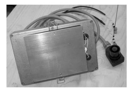
There are no extra surface thermocouples on the flat plate that require connection unless the unit is being used with the optional Data Acquisition Upgrade HC351A and this is dealt with in a separate manual. The flat plate is located in the open section of the tunnel and secured with the two toggle clamps. Ensure that the heater is located in the tunnel with the power connection at the top as shown on page 1
