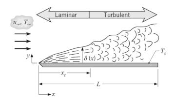
The heat lost due to forced convection can be determined from
