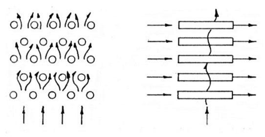
Various tube and fin layouts have been devised in order to improve the efficiency heat exchangers and thereby reduce the physical size for a given heat transfer rate. However, the objective of all of the arrangements is to promote turbulence in the fluid flowing across the extended surfaces.
