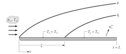
Velocity boundary layer growth begins at x = 0, while thermal boundary layer development begins at  $x = \xi$ . Hence there is no heat transfer for  $0 < x < \xi$ . Therefore, we apply a correction to Nu number.
