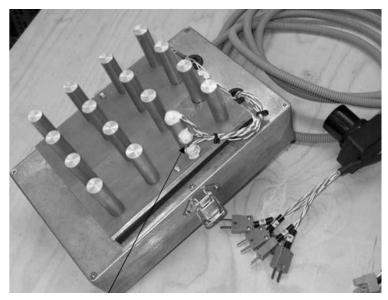
There are three extra thermocouples on the pins (T2, T3, T4) that require connection to the control console extra sockets. These are fitted with thermocouple plugs (shown above) that match the sockets on the console. The pinned plate is located in the open section of the tunnel and secured with the two toggle clamps. Ensure that the heater is located in the tunnel with the power connection at the top as shown on page 1
