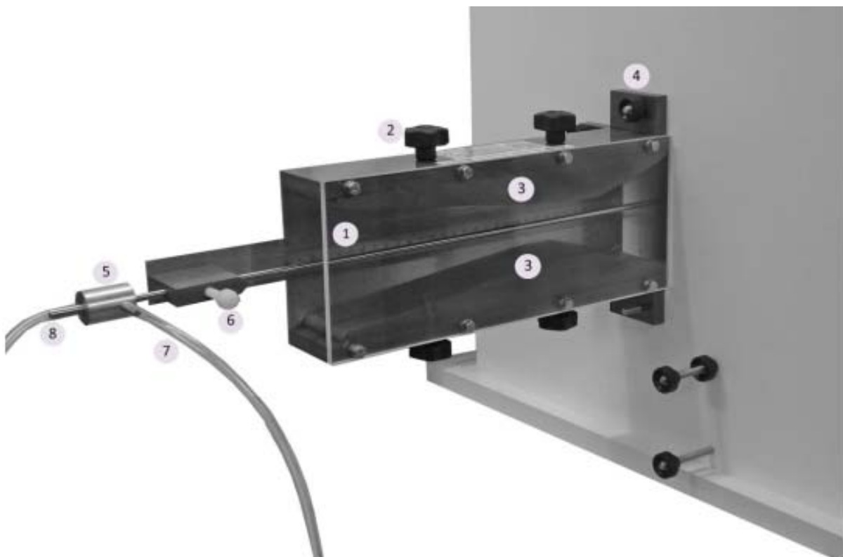
General experimental setup of Multi-Tube Manometer: 1. Position Measuring Scale; 2. Profile Retaining Nuts; 3. Duct Profiles; 4. Mounting Nuts; 5. Pitot-Static Tube; 6. Locking Nut; 7. Static Pressure Tapping; 8. Total Pressure tapping
