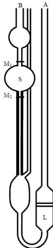
Figure 4. Ostwald viscometer. Is measured the time that use the liquid going from level M2 to M1.
